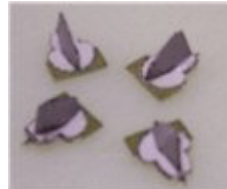
glued finished vanes attached to roots
