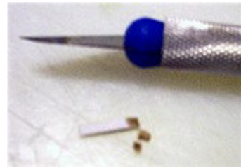
cutting the bevel into the insert
