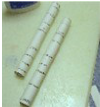
the 2 engine tube halves 1 with coupler inserted
