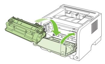
If no paper was jammed inside the print-cartridge door, open the jam-release door at the back of the product.
