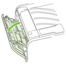
Media guides ensure that the media is correctly fed into the printer and that the print is not skewed (crooked on the media). When loading media, adjust the media guides to match the width of the media that you are using.
