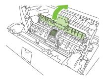
4. Press the two black retaining tabs outward until the pickup roller is released from its seat.
