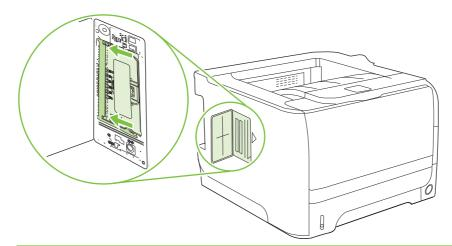
NOTE: To remove a DIMM, first release the locks.
