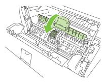
**11.** Reinstall the print cartridge, and close the print-cartridge door.
