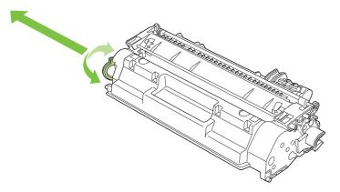
5. Align the print cartridge with the tracks inside the product, insert the print cartridge until it is firmly seated, and then close the print-cartridge door.
