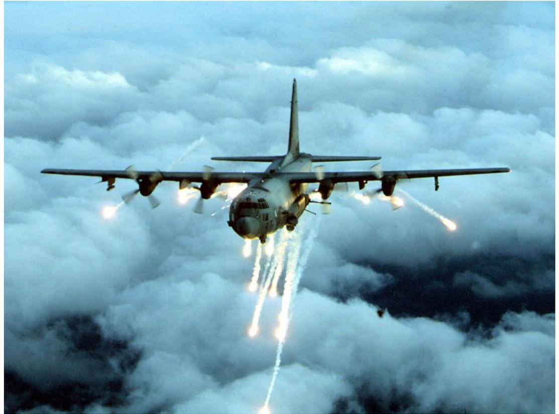
The AC-130U was armed with a 25mm Gatling-gun (capable of firing 1800 rounds per minute), a single-barrel, rapid-fire 40mm Bofors cannon, and a 105mm Howitzer. The AC-130U replaced the two 20mm cannon used on the AC-130H with one trainable 25mm cannon while retaining the other weapons. The AC-130U employs the latest technologies and can attack two targets simultaneously.
