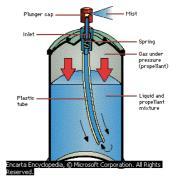
valve allows the product to be forced up a tube and through the valve. The liquefied gas in the bottom of the container vaporizes to keep the pressure constant.
