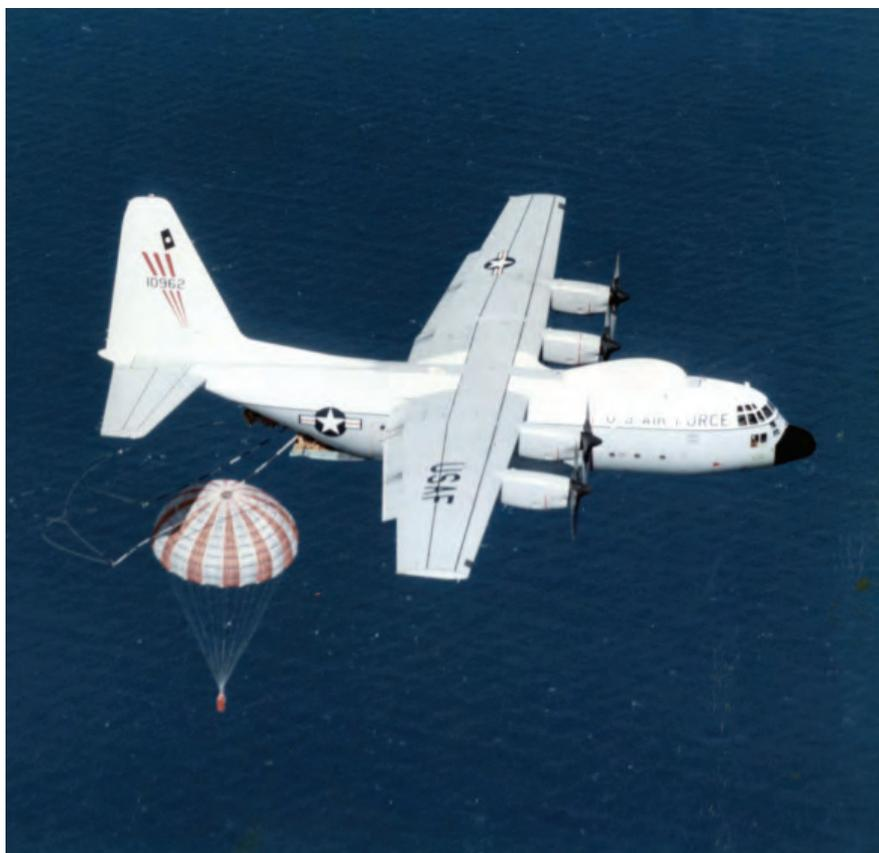
A modified JC-130 Hercules captures a GAMBIT film bucket with hooks trailing behind and below the aircraft. (Undated photo courtesy of Randy Chang.)
