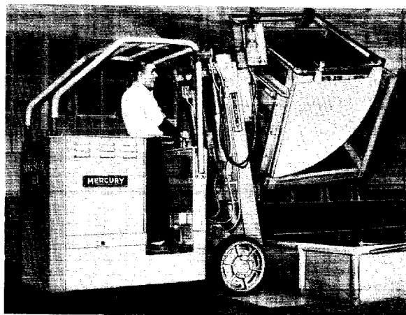
Rotating Fork Carriage: Mercury "Yank" equipped with a "Roto-Lift" carriage which revolves 180 degrees in either direction to permit dumping of loads, upending of rolls, etc.
