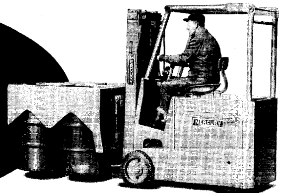
Drum Handler: Tray-Hart hydraulic drum carrier with a capacity for handling 55 gallon drums. Illustration shows drum carrier installed on a model A-3444, 3000 lb. "Jeep" fork truck chassis.
