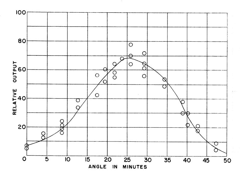
RELATIVE OUTPUT OF 0.53 MICRON RADIATION FUNCTION OF CRYSTAL ALIGNMENT TO 1.06 MICRON INPUT BEAM
