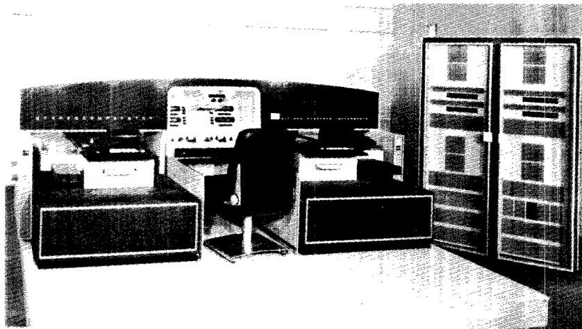
FIGURE 8. High-precision stereocomparator developed under NPIC R&D program and currently being manufactured by Houston Fearless Corp. Calif.
