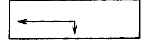
FIG. 4 — Channel Facility allowing information from either direction to be turned and fed to spur station.
