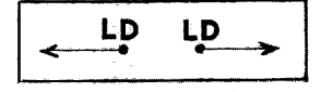
FIG. 2 — Channel access on a private line basis to allow transmission and reception of information in one of two directions . . . one facility required, or transmission and reception of two pieces of information in opposite directions . . . two facilities required.
