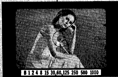
The match-needle viewfinder: just align two indicators for correct exposure. Because you're doing some of the work, you can save some money.
