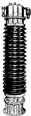
Fig. 32 - Type VTO/TVE 150 voltage transformer - 150 kV 150.000/V \sqrt{3} / 100/V \sqrt{3} - Class P 200 VA, class Q 300 VA.
