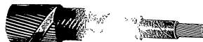
34a) Type: TPF single-core or multicore Conductor and insulation: see type no. 34. Protective covering: round or flat steel wire armoured. Recommended for: mining installations, tunnel hydraulic power conduit, mines.
