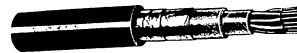
40) Type: TTPR Polythene local telephone cable, plastic jacket. Conductor: plain copper wire. Insulation: coloured polythene.
