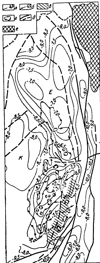
Fig. 1. Structural map of the surface of the substructure of the Yenbek-Zharkamys region: \alpha --isohypses of the surface of the substructure, km; \beta --isohypses for stratum P_3 ; \theta --Tobusken arch; \varepsilon --local subsalt upheavals; \delta --tectonic disturbances; e --Uraltau zone; E --Yenbek ridge; K --Zharkamys ridge; K --Kzyldzhar ridge
