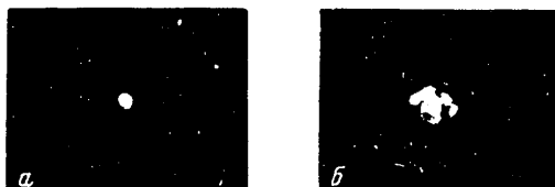
Figure 3.18. Photograph of the light source (a) and its image (b) created by mirror No 9.
