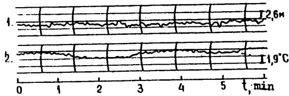
Figure 4. Fragment of Depth (1) and Temperature (2) Signal Recordings at a Fixed Horizon in the Thermocline
