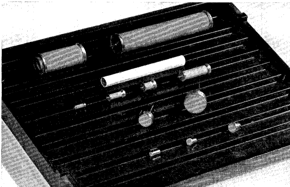
Some L cathodes (with a cigarette for comparison of size). The L cathode has a porous, metal, emitting surface and can withstand heavy loads, say 100 A per cm 2 .
