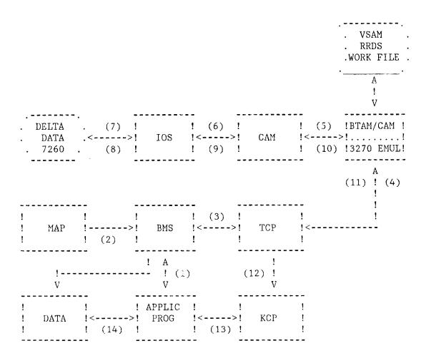
As in the previous two sections the structure of CICS software has been kept as original as possible. Modifications for unsupported terminals (ie DELTA DATA 5260) have been made in the form of programs written under or along side of CICS. It is our intent to follow similar guidelines using the available ALLSTAR system and incorporate the functions of a modified BTAM/CAM interface to achieve our goal of 3270 emulation using the agency standard DELTA DATA 7260 terminal.
