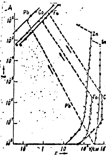
Fig. 1. Volt-ampere characteristics of structures in Po, Fe, Co, Zn and Sn powders (broken lines indicate breakdown leading to the formation of a bridge).
