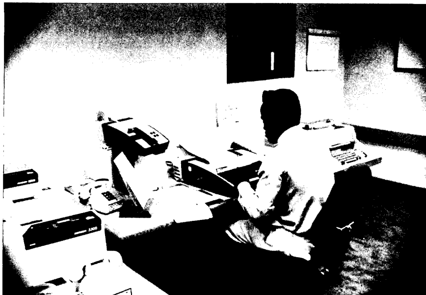
FIGURE 5-1. MESSAGE CENTER COMMUNICATIONS EQUIPMENT: OPERATOR USING FEMA NATIONAL TELETYPE SYSTEM (FNATS) MACHINE
