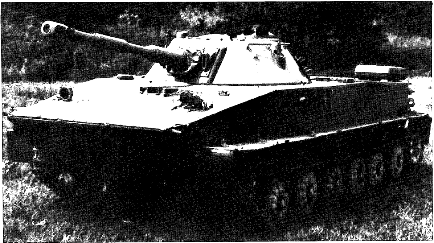
The PT-76 weighs 14 metric tons and has a 76-millimeter gun. This fully amphibious tank uses water jets for propulsion when in water. The Soviets provided the Sandinistas about 30 of these light tanks in 1984.
