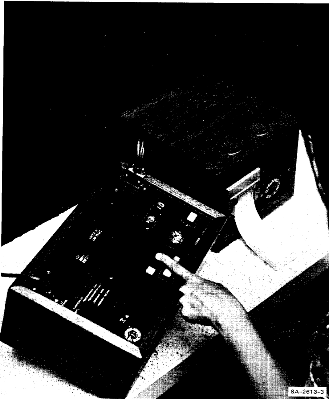
FIGURE 19 FOUR-STATE RANDOM TARGET GENERATOR USED IN THIS EXPERIMENT An incorrect choice of target is indicated. Two of the five "encouragement lights" at the top of the machine are illuminated. The printer to the right of the machine records data on fan-fold paper tape.
