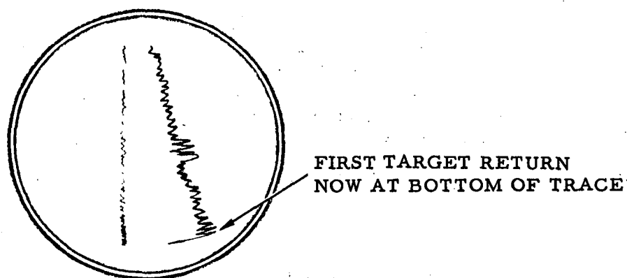
FIG. 4-26 APQ-56 MONITOR SCOPE TRACES - ALTITUDE SETTING CORRECTED - AIRCRAFT IN RIGHT BANK
