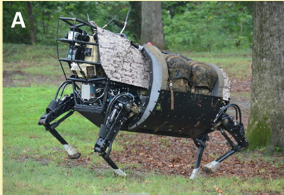
A. The Defense Advanced Research Projects Agency (DARPA)-funded BigDog robot uses four animal-like legs to traverse terrain too rough or slippery for conventional vehicles. It is also capable of recovering its “balance” if it slips. The current iteration of the program, the Legged Squad Support System (LS3) (above) seeks to demonstrate that a highly mobile, semiautonomous legged robot can carry 400 lbs. of load through rugged terrain. 6
