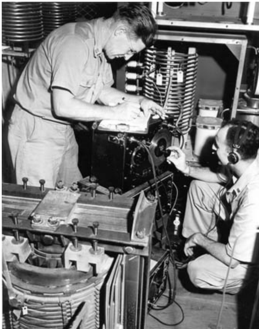
OWI personnel adjusting the KSAI radio transmitter to new frequencies to avoid jamming by Japan
